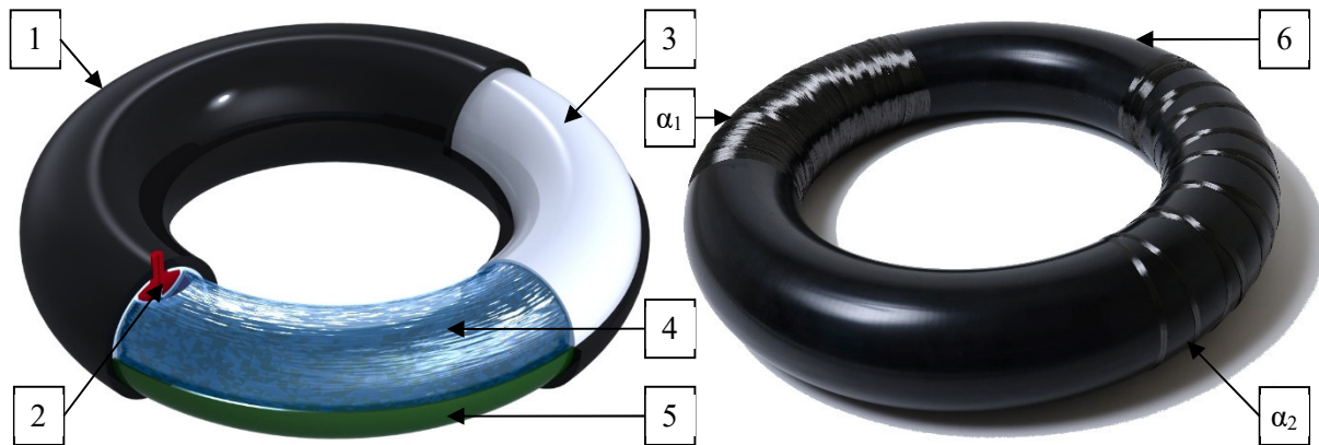
Figure 6: CAD design of TCPV type LSE 1.4 (left) and winding demonstrator with PU liner (right)
