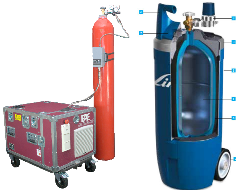
Figure 1: left: Fuel cell operated mobile power generator of FAE Elektrotechnik GmbH & Co. KG with 1 kW constant electrical output and a standard steel bottle (filling volume 8.9 m 3 , filling pressure 200 bar, weight 80 kg), right: GENIE® bottle (filling volume 5 m 3 , filling pressure 300 bar, weight 32.7 kg) of Linde AG ( www.linde-gas.com/genie )
